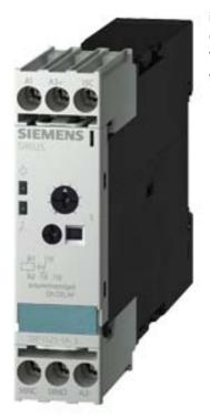
Timing relay, electronic Phase-out product! For further information, contact our sales department ON delay 1 CO contact 15 time ranges 0.05 s...100 h 24, 200...240 V AC and 24 V DC at 50/60 Hz AC with LED, screw terminal
